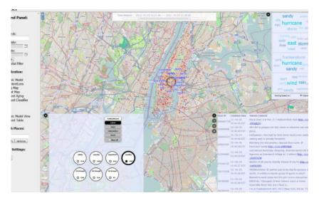
SMART system includes a map view, a topic view, a stream classifier view, and a message table. The classifier view loads traffic, severe weather and safety classifiers. Clicking the severe weather related classifier, other linked views refresh to show corresponding data. Content lens in the map view visualizes keywords extracted from tweets in the Manhattan area.
